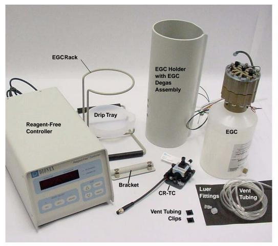
Figure 83. RFC-30 Components
