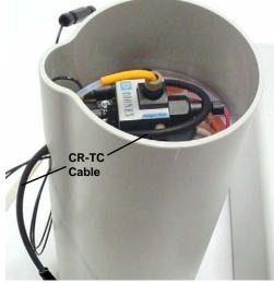
Figure 89. Installing the CR-TC
