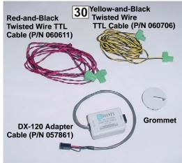
Figure 63. DX-120 TTL Cables
