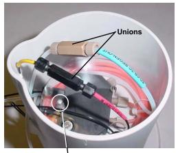
Metal stud for mounting the CR-TC Figure 85. EGC Holder (upside down)
